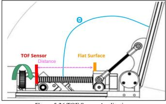
Figure 5.26 TOF Sensor Application
