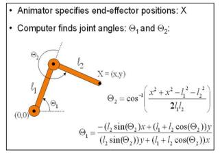
Figure 5.8 2D Inverse Kinematic Nonlinear Equations
