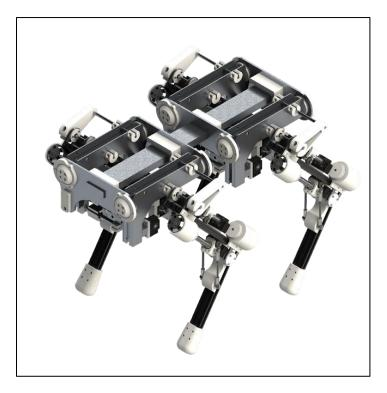
Figure D1.2. Large-Scale Dog CAD Model (Side-View)
