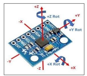
Figure 5.25 A look into the MPU6050 and the different readings it takes at different axes.
