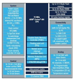
Figure 5.6. STM32 Cortex M4 Specifications
