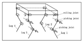
Figure 3.2 Small Model Joint Placement Diagram
