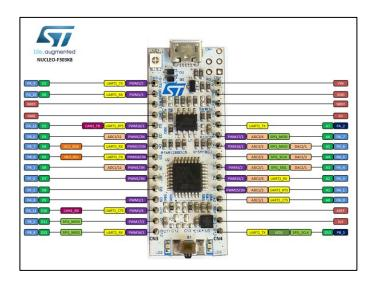
Figure 5.7 STM Nucleo Board Pinout
