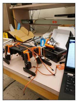
Figure 5.4 3D Printed Small Scale Dog Model
