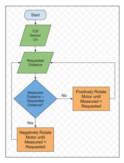
Figure C1.1. TOF Sensor Feedback Flowchart
