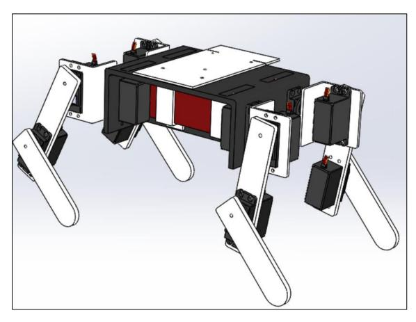
Figure D1.7. Small-Scale Dog CAD Model
