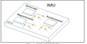
Figure 5.23 9DOF IMU
