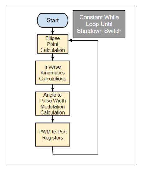
Figure C1.3. Small-Scale Dog Software Block Diagram
