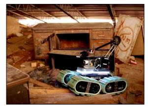
Figure 2.11. KOHGA3 Ground Robot for Search and Rescue and Vacant Building Inspection
