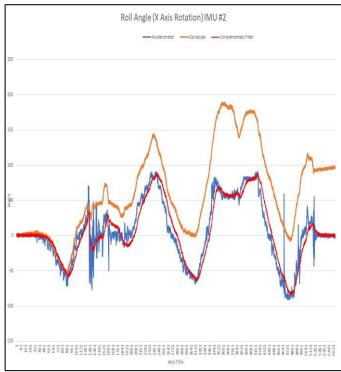
Figure 9.4 . IMU #2 X-Axis Rotation Filtered versus Unfiltered
