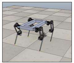
Figure 5.3 Diagram representation of our 12 Servo Dog
