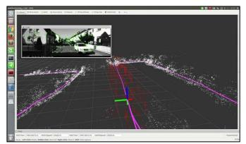
Figure 5.21 ORB-SLAM2 Point Cloud Map Example
