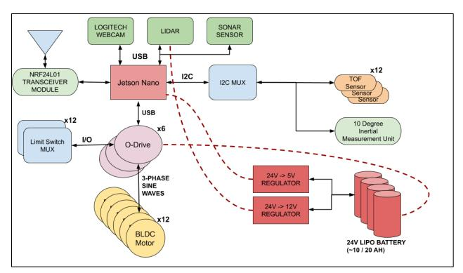
Figure B1.1. Large-Scale Dog Hardware Block Diagram
