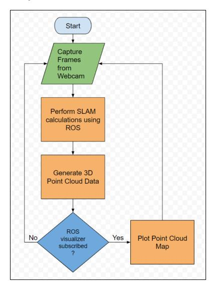
Figure C1.2. ORB-SLAM2 3D Point Cloud Flowchart
