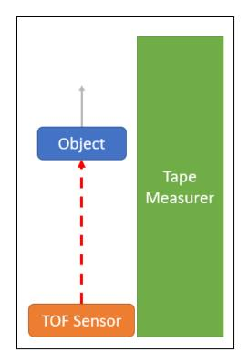
Figure B1.3. Time-of-Flight Testing Procedure (Top-View)
