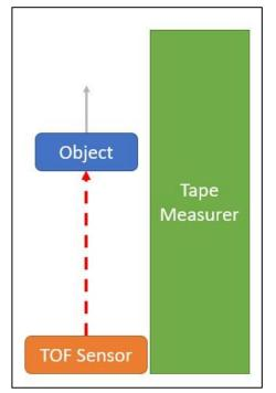
Figure 9.7 TOF Sensor Testing Procedure (Top-View)
