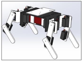
Figure 3.1 Small Scale CAD Model of Robotic Dog Source: Please refer to [6]
