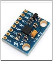
Figure 9.1 MPU6050 IMU Source: Please refer to [4]
