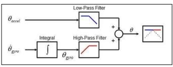
Figure 5.24 IMU Angular Velocity Calculation Process
